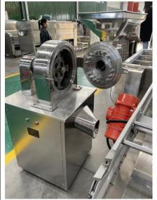
Capacity: 50-100 kg/h Fineness: 20-120 mesh Cutter diameter: 200 mm Main Power: 4.0 kw Machine Weight: 140 kg
