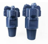
It is an ideal drill bit to use in sandstones limestones and in the transition from heavily weathered crystalline rocks into the consolidated fresh underlying rock to drill pockets to set surface casing to allow drilling to switch to compressed air and DTH down The Hole hammer and percussive button bit.
