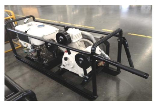
PAT release new 'Borehole Development Compressor unit', powered by monocycle diesel engine 10 HP, heavy duty type, high torque, and very save fuel consumption,
