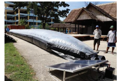
Solar bubble dryer Credit: Brian Atkin
