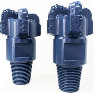
It is an ideal drill bit to use in sandstones limestones and in the transition from heavily weathered crystalline rocks into the consolidated fresh underlying rock to drill pockets to set surface casing to allow drilling to switch to compressed air and DTH down The Hole hammer and percussive button bit.
